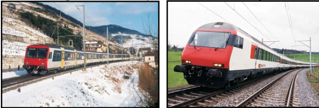
Figure 10. Electric Multiple Unit Vehicles with Catenary
