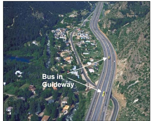
Photo simulation of the Bus in Guideway alternative in the median in Lawson.
