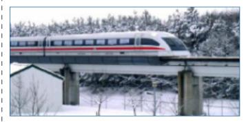
Transrapid is German developed system, commercially available in Shanghai, with a lower cost than steel-wheel trains with tunnels. Also, it can climb steeper (7%) grades.
