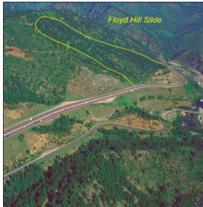
The terrain on the east side of Floyd Hill consists of rolling hills. Rock is not mineralized and ranges from good to poor quality, with a number of major and minor faults (Reed et al. 1973). Rock excavations along US 40 through Mount Vernon Canyon generate rockfalls that affect US 40 and occasionally I-70. Isolated areas in these road cuts have generated larger, more troublesome rockslides. Some slides have been large enough to close US 40 for extended periods of time.
