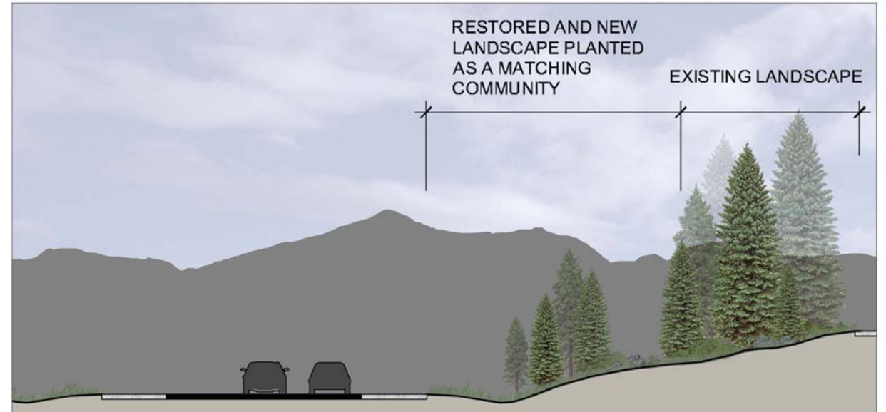
A | Areas of disturbance should be restored using a mixture of native landscape plants, rocks, stumps, and other natural materials to mimic and blend with the existing surroundings.
