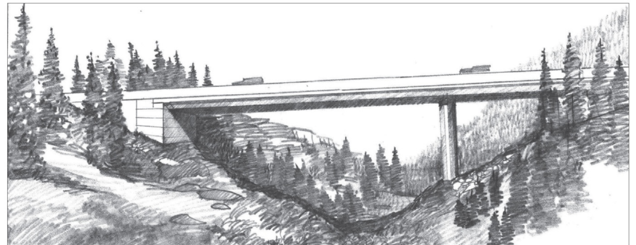
C | Open bridge solutions span significant landforms and stream corridors and leave undisturbed drainages below, minimizing environmental disturbance and impacts to the hydrologic and visual characteristics of the watershed.
