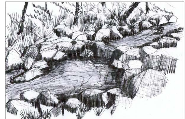
D | Drop structure using indigenous rock construction.
