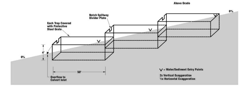
I-70 Sediment Control Action Plan Typical Below-Grade Sediment Traps 6% Shoulder Grade
