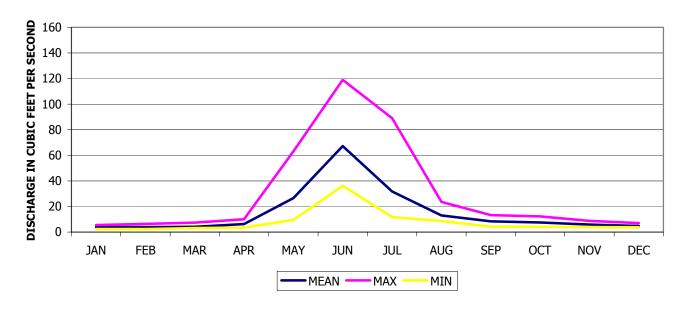
STRAIGHT CREEK MONTHLY MEAN DISCHARGE Below Laskey Gulch Near Dillon, CO 1987-2000 Drainage Area = 18.3 sq-mi
