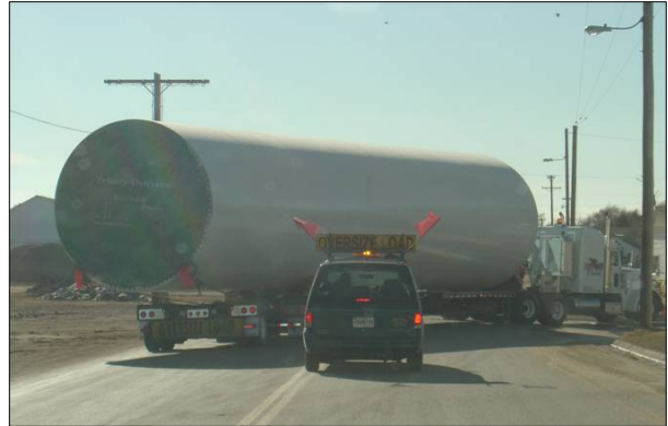
Picture 2.4: Wind turbine tower segment at 90-degree turn westbound to northbound in Cheyenne Wells
