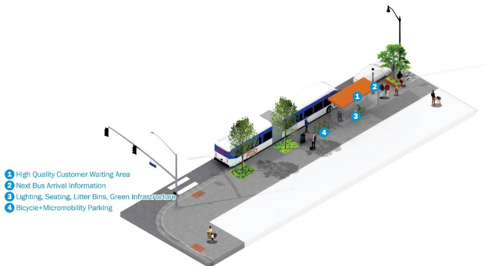
Figure 8-3: Recommendation – Speed and Reliability Example Stop Improvements
