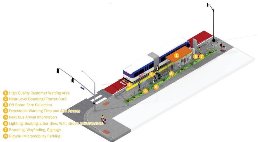
Figure 8-6: Recommendation – Side-Running BRT Example Station
