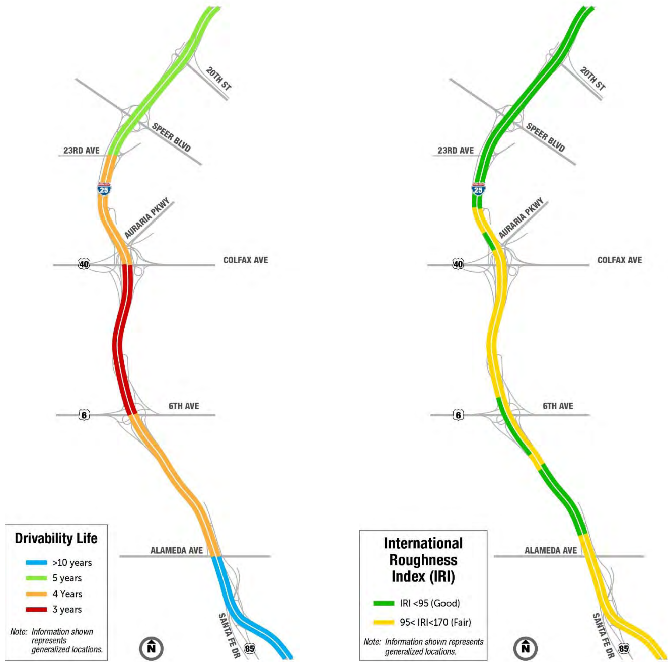
Figure 32. Remaining Pavement Drivability Life and IRI Rating
