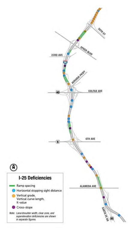
Figure 2. Ramp Existing Geometric Deficiencies (20th Street to Santa Fe Drive)
