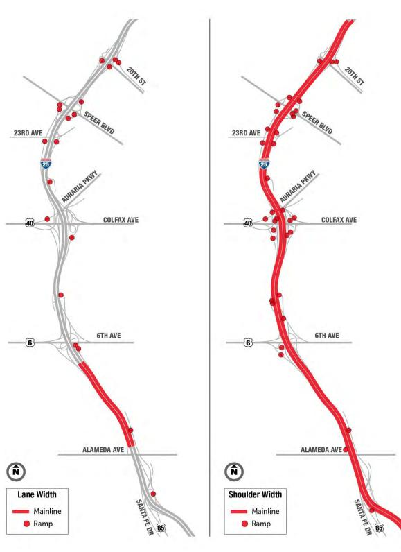
Figure 3. Existing Lane and Shoulder Width Deficiencies (20th Street to Santa Fe Drive)
