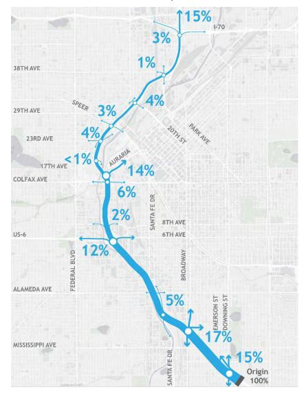
Figure 2: Northbound I-25 Traffic from Downing Street to Northbound Off-Ramp Destinations
