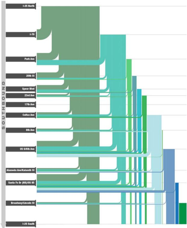
The width of the lines in this figure are scaled based on total daily traffic volumes. The vertical portion of each line represents traffic coming onto I-25 from an interchange. The horizontal portion of the line represents the portion of traffic exiting to each interchange.
