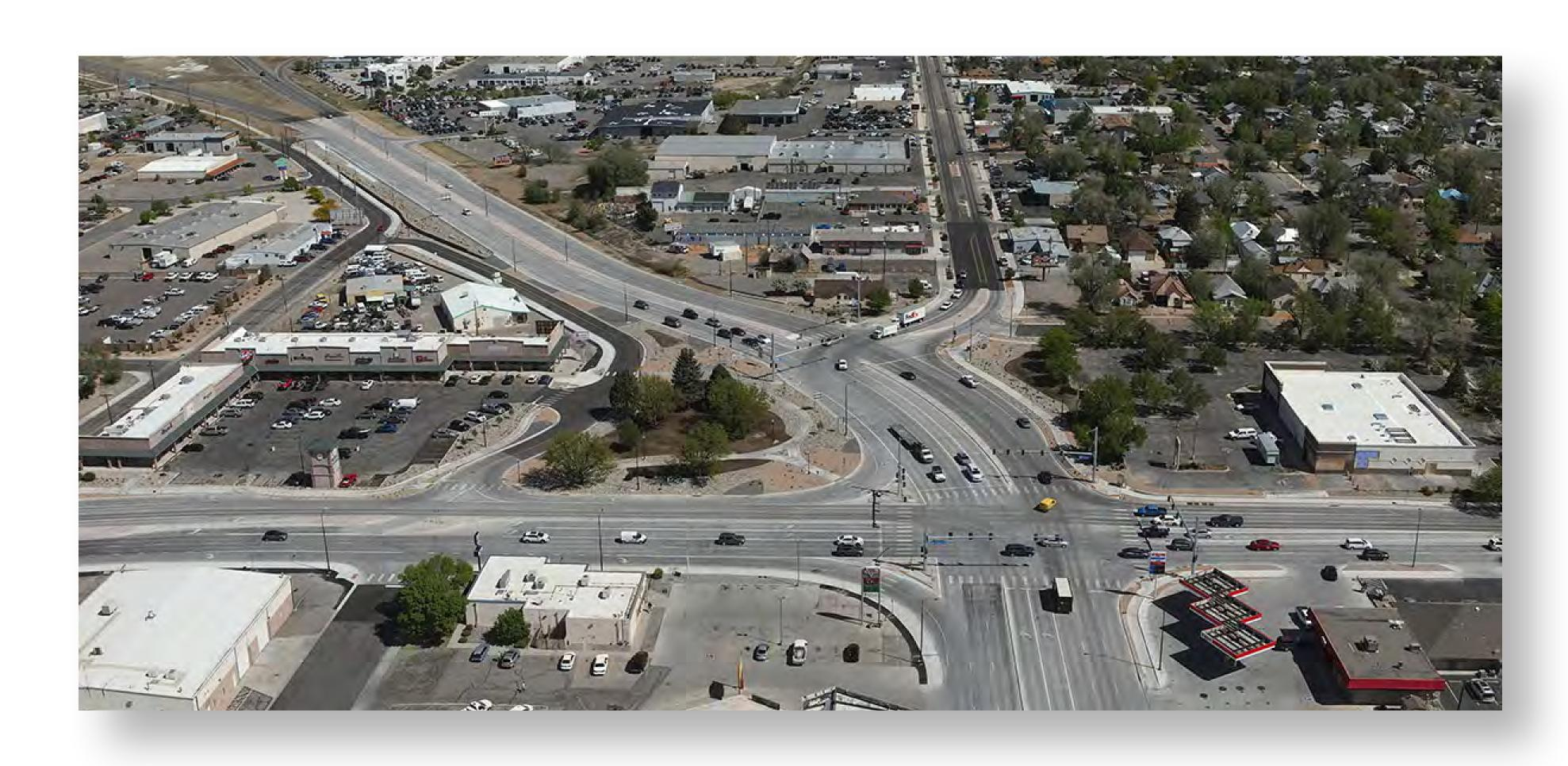
Much of the major project work for Phase 5 was completed during the 2021 construction season. Work in 2022 included hot mix asphalt paving, curb, gutter, and sidewalk as well as final landscaping and striping.
