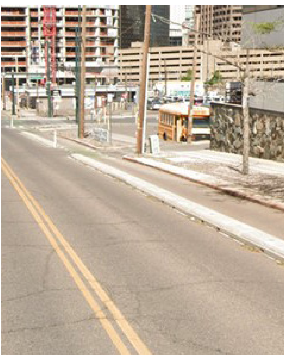
Continuous concrete curb-protected bike lane.
