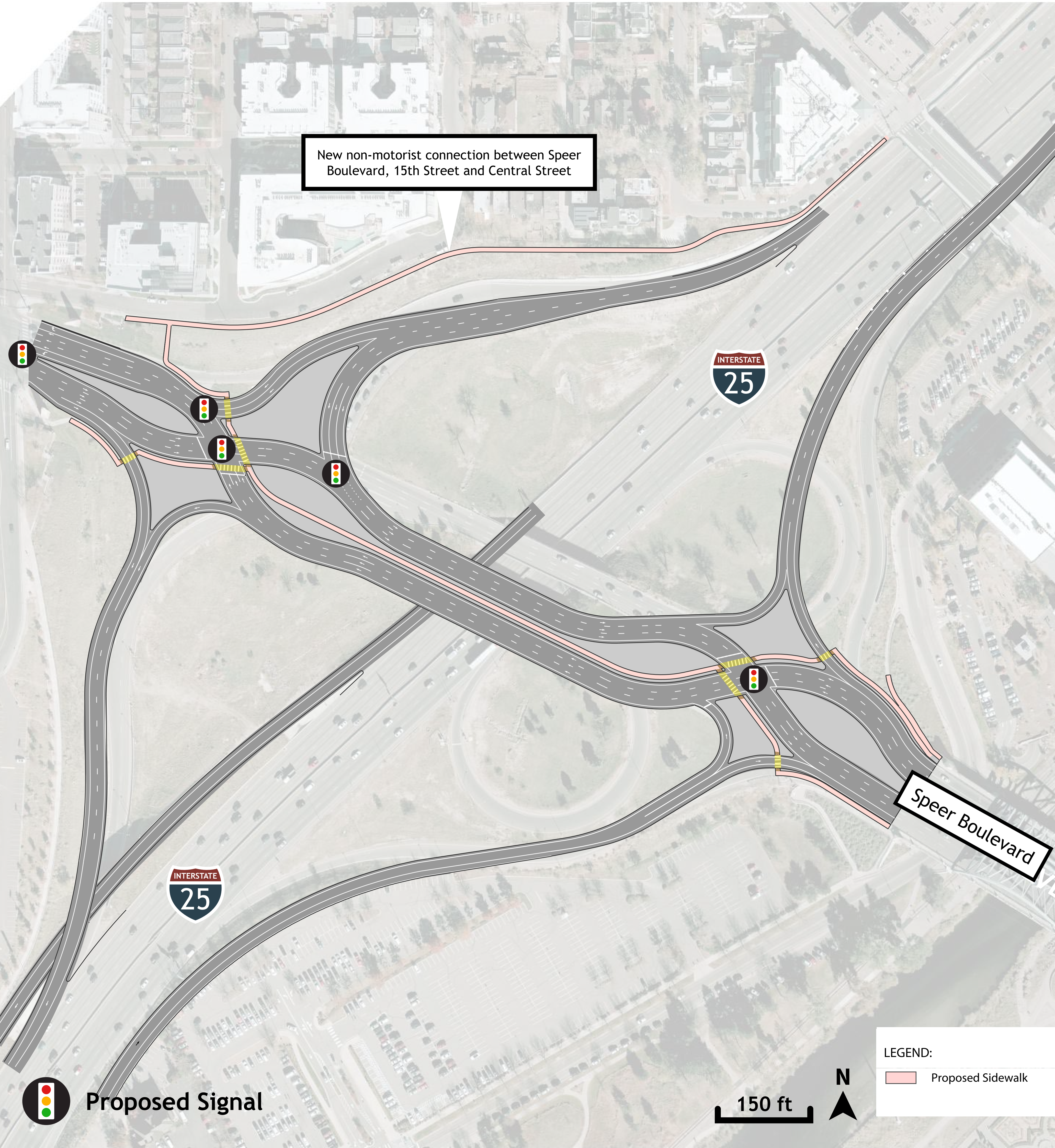
Map showing the recommended diverging diamond design configuration alternative near the 23rd Avenue and I-25 interchange.
