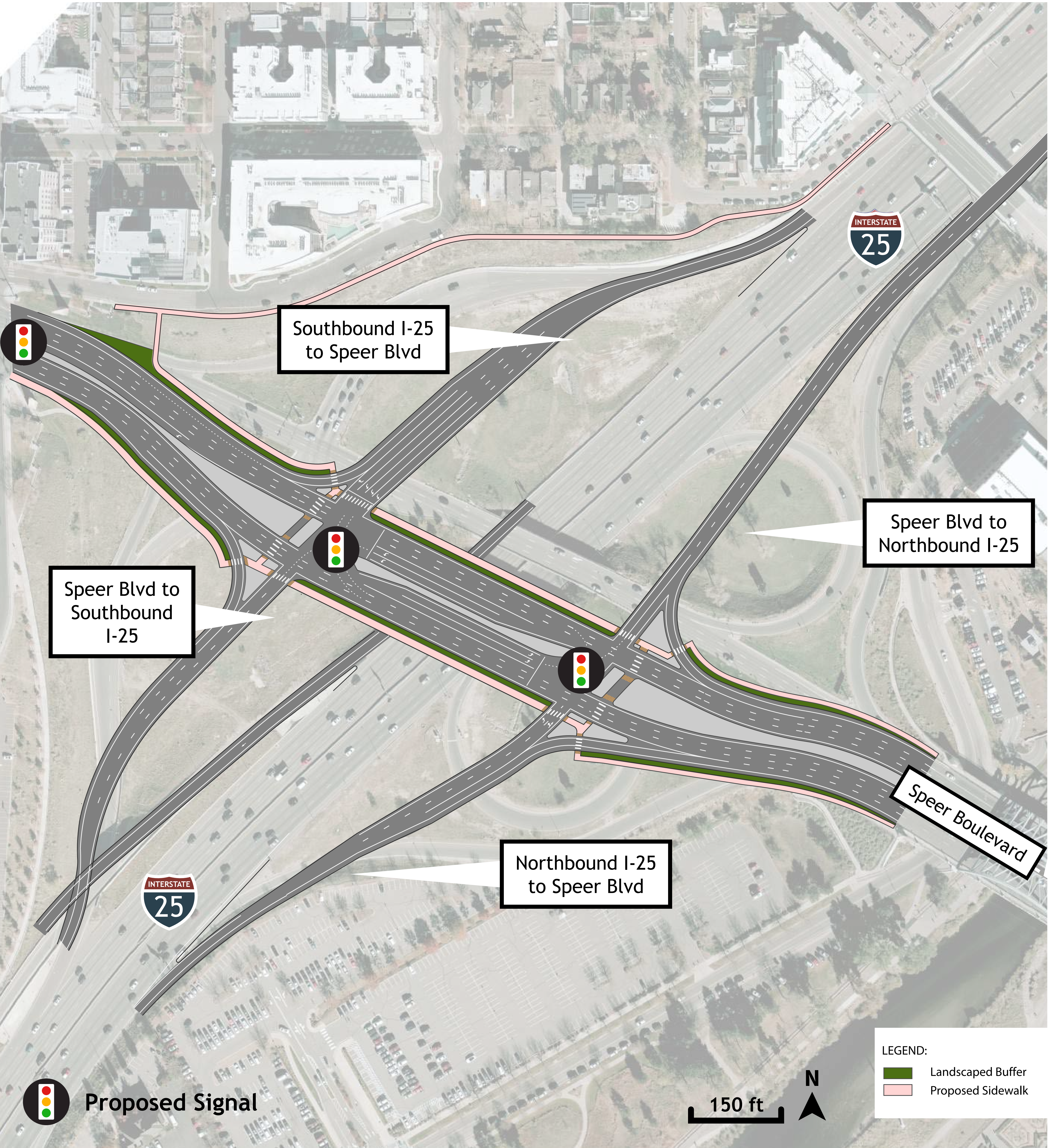
Map showing the diamond design configuration alternative near the Speer Boulevard and I-25 interchange.
