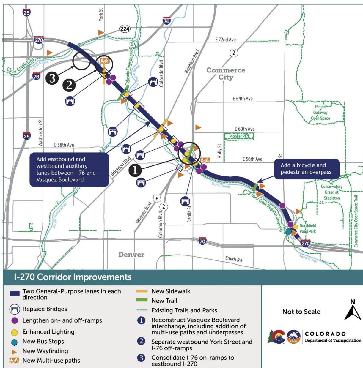
Figure 14. Minimal Build Alternative
