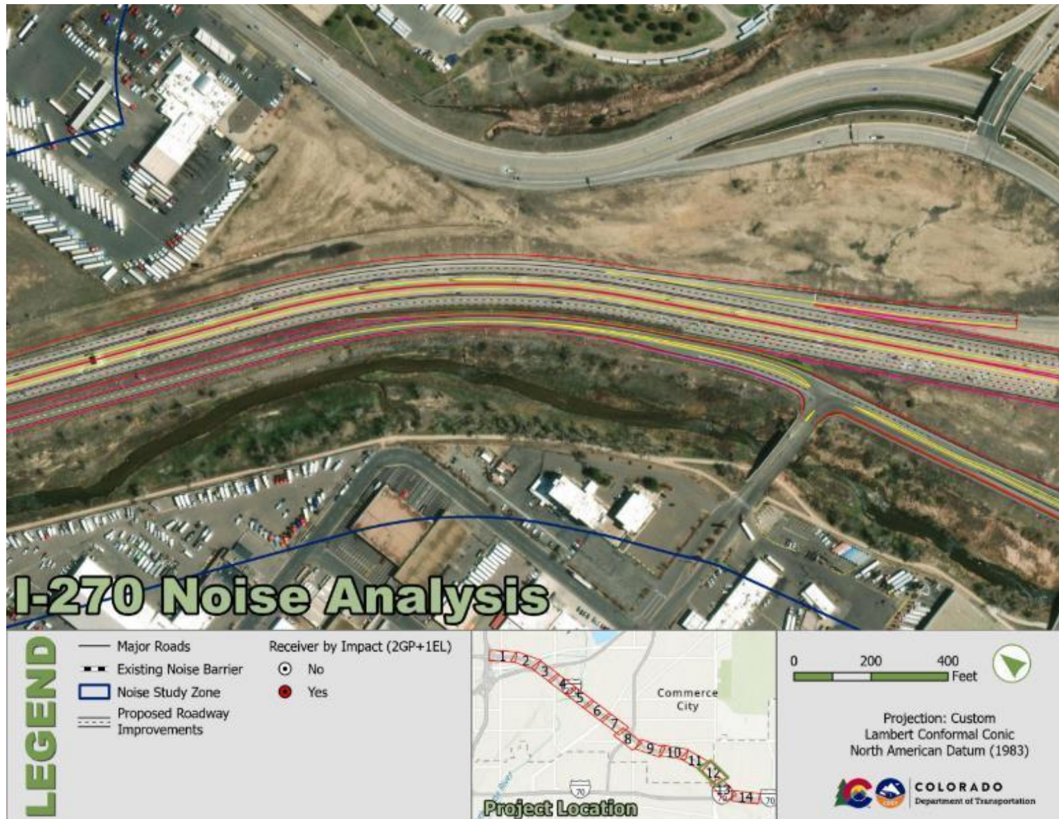
Figure 54 Roadways and Receiver Noise Levels for Design Year (2050) EL Build Alternative (Impacts Identified)
