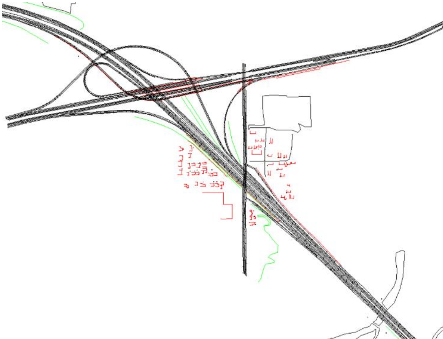
Figure 4 TNM Model Objects for Design Year (2050) GP Build Alternative
