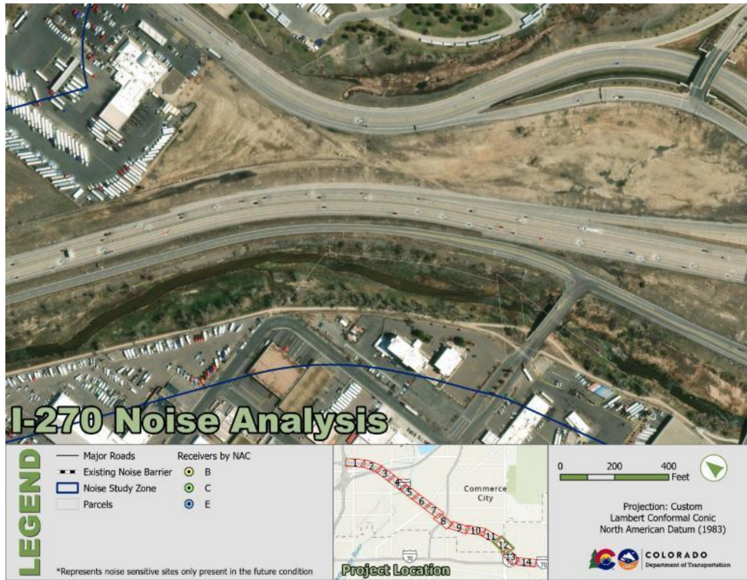
Figure 26 Roadways and Receiver Locations for Existing Condition (2023) and Design Year (2050) No Action Alternative
