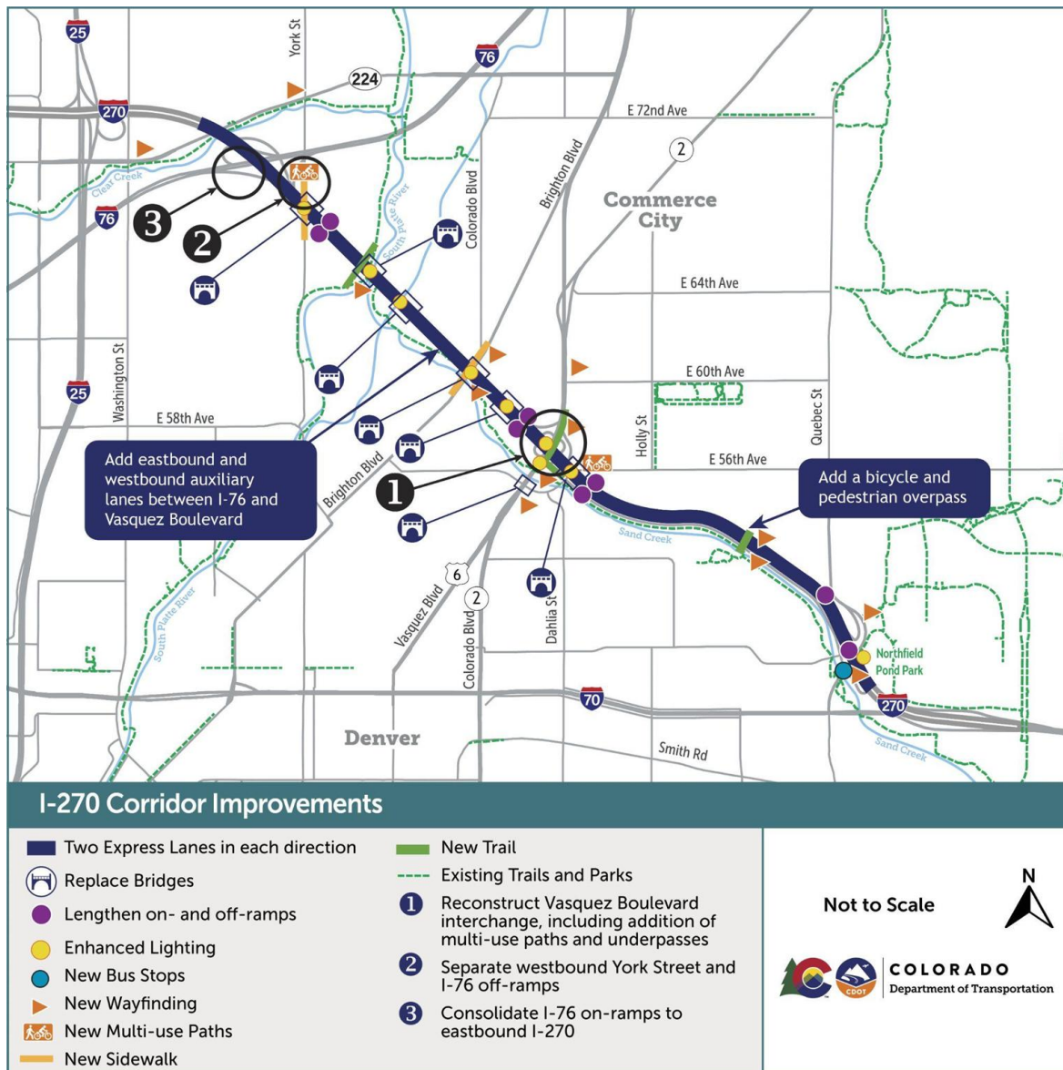
Figure 2. Two Express Lanes that Accommodate Transit Alternative
