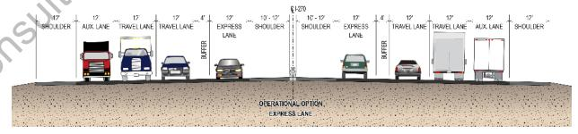
Figure 2-2. Typical Roadway Section with Auxiliary Lane
