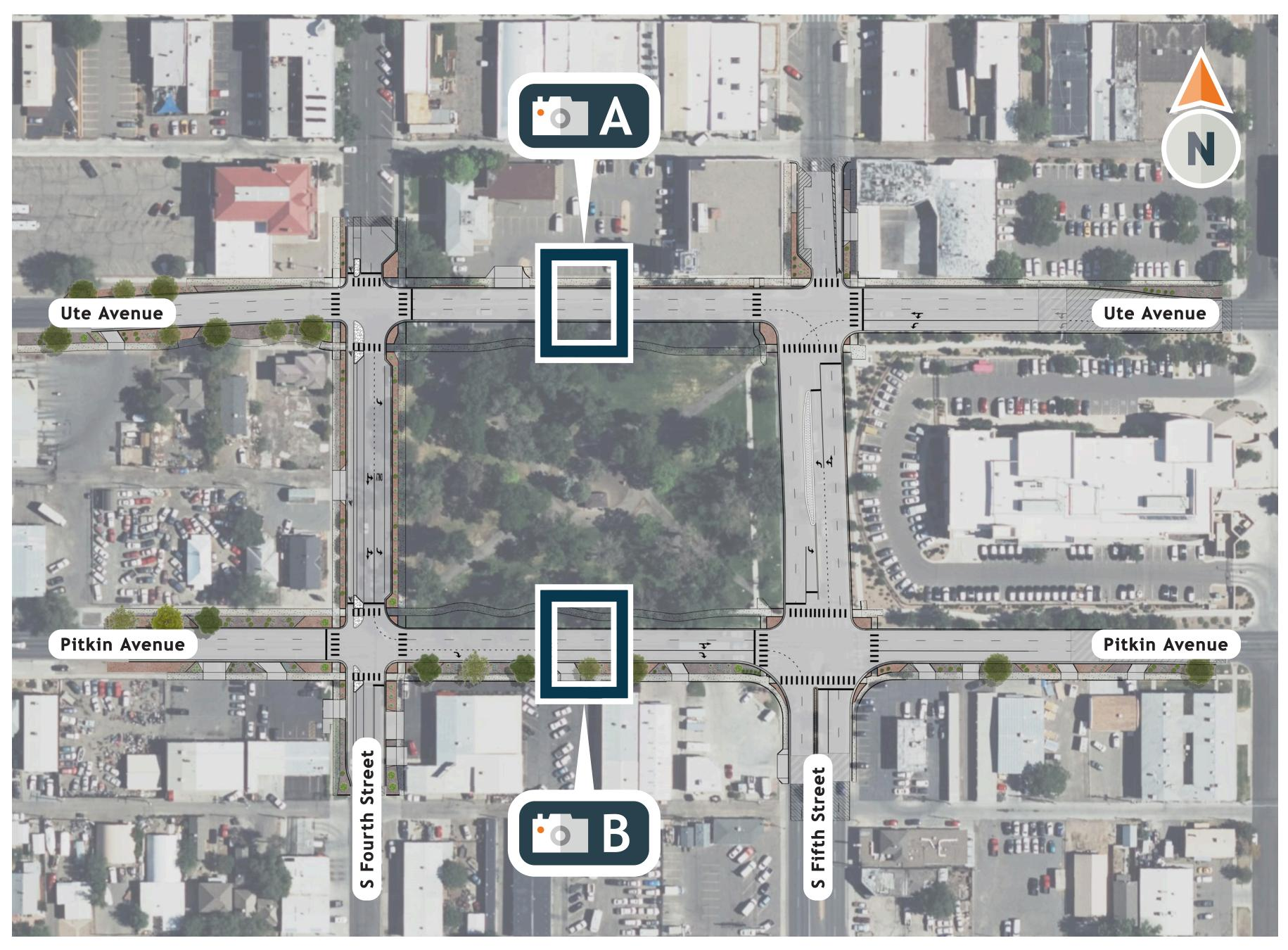
Map showing the Phase 7 Final Design Improvements from approximately Third Street to Sixth Street. Planned upgrades include three 11-foot lanes on Ute and Pitkin Avenues, 6- to 8-foot sidewalks, 2- to 11-foot landscaped buffers, and new concrete pavement. Side street updates include asphalt on Fourth Street and mostly concrete on Fifth Street, with exceptions north of Ute Avenue.
