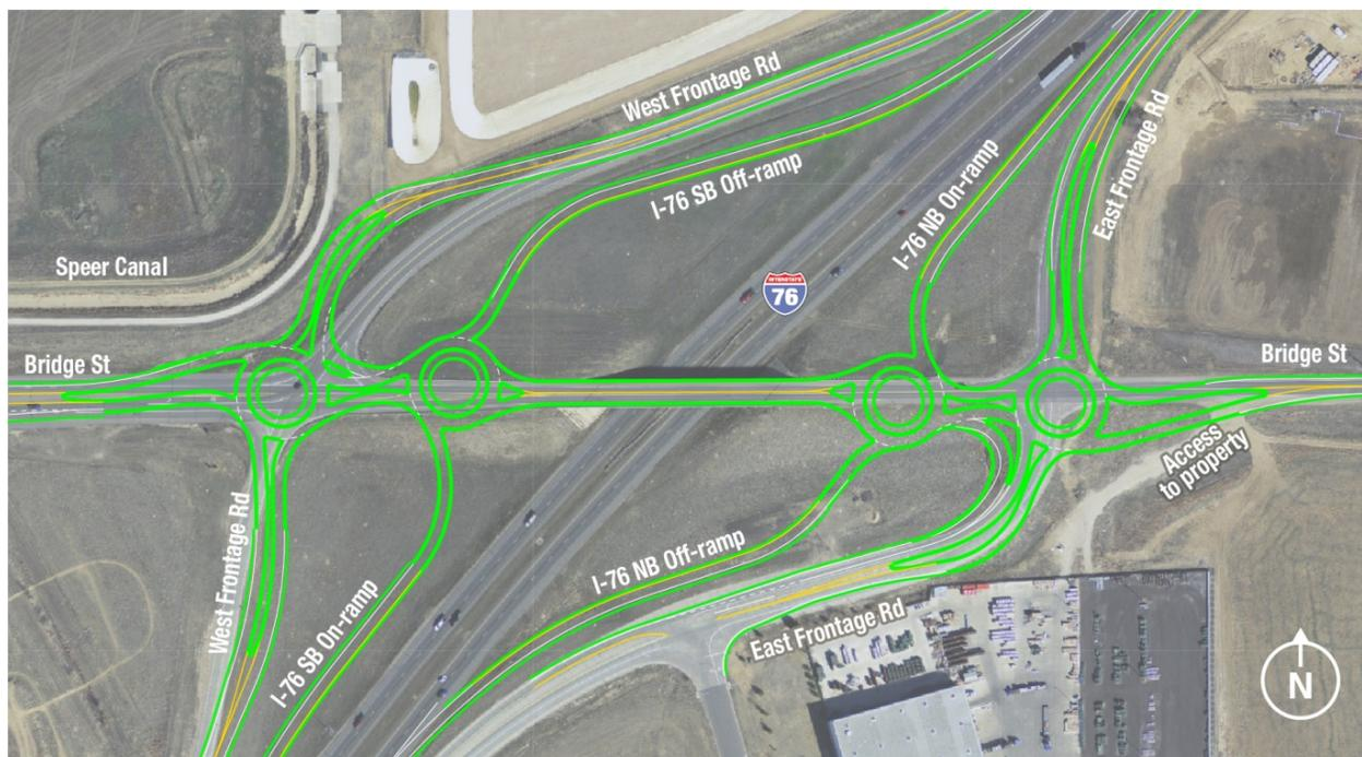
**Exhibit 3-8. Conceptual Design and Traffic Movement Pattern of Alternative 2**
