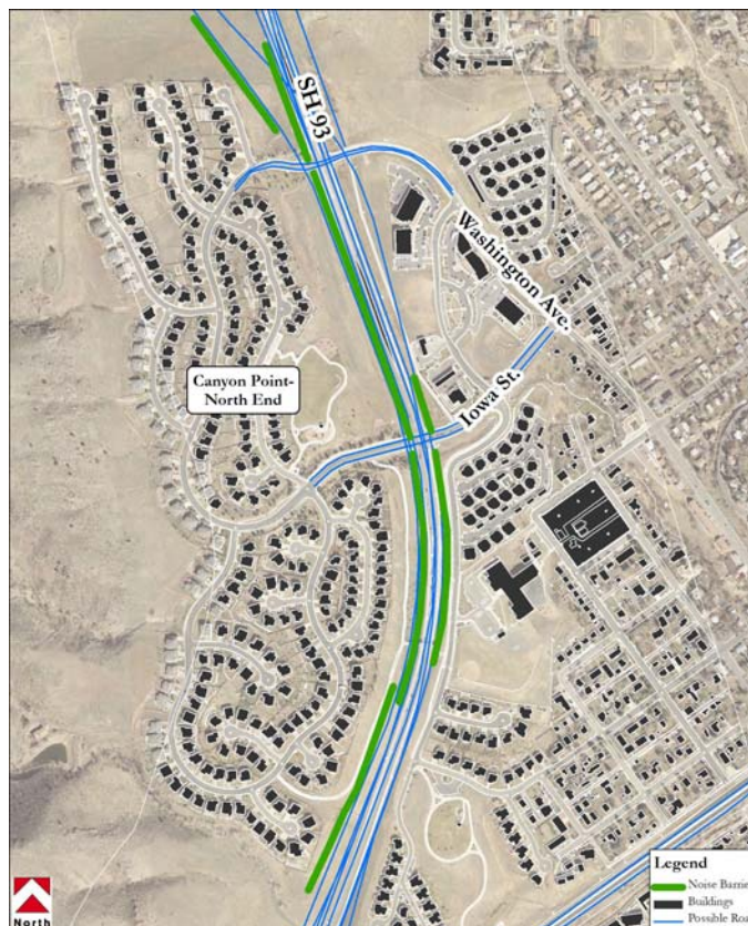
Figure 4.7-16 Recommended Noise Barriers near Canyon Point
