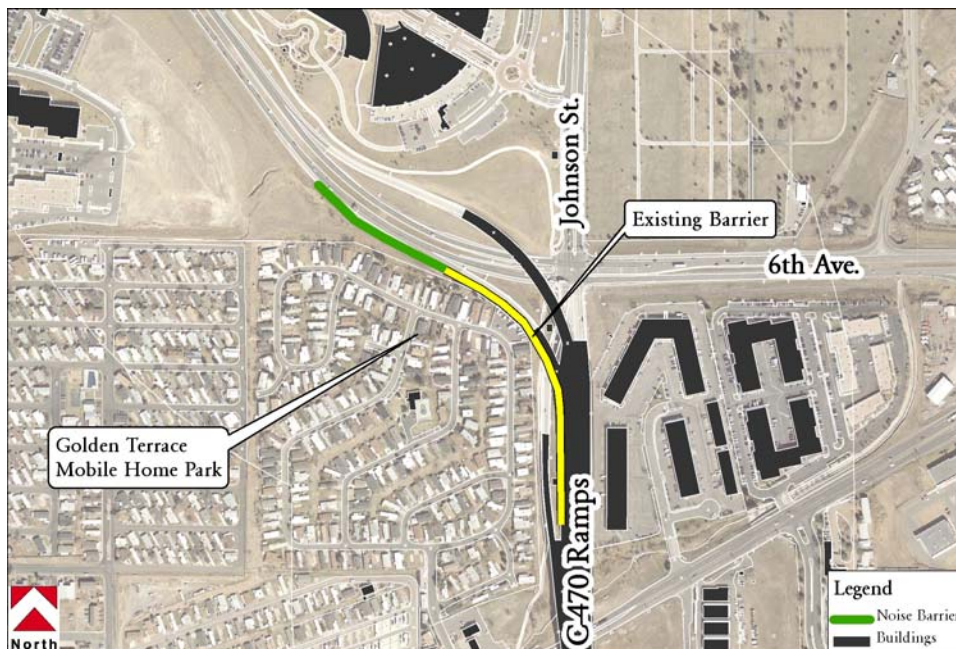
Figure 4.7-18 Recommended Noise Barrier near Golden Terrace
