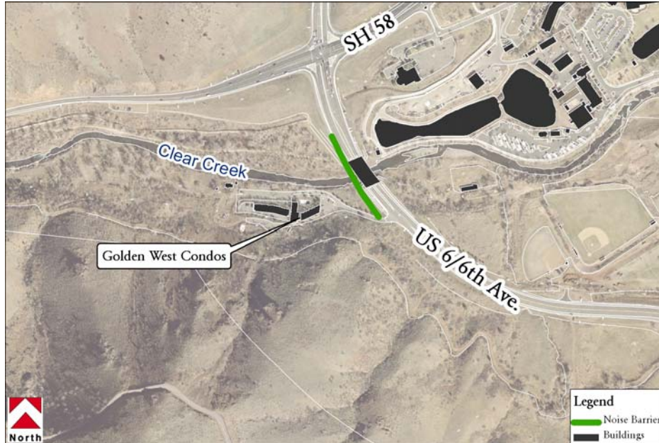
Figure 4.7-17 Recommended Noise Barrier near Golden West Condos
