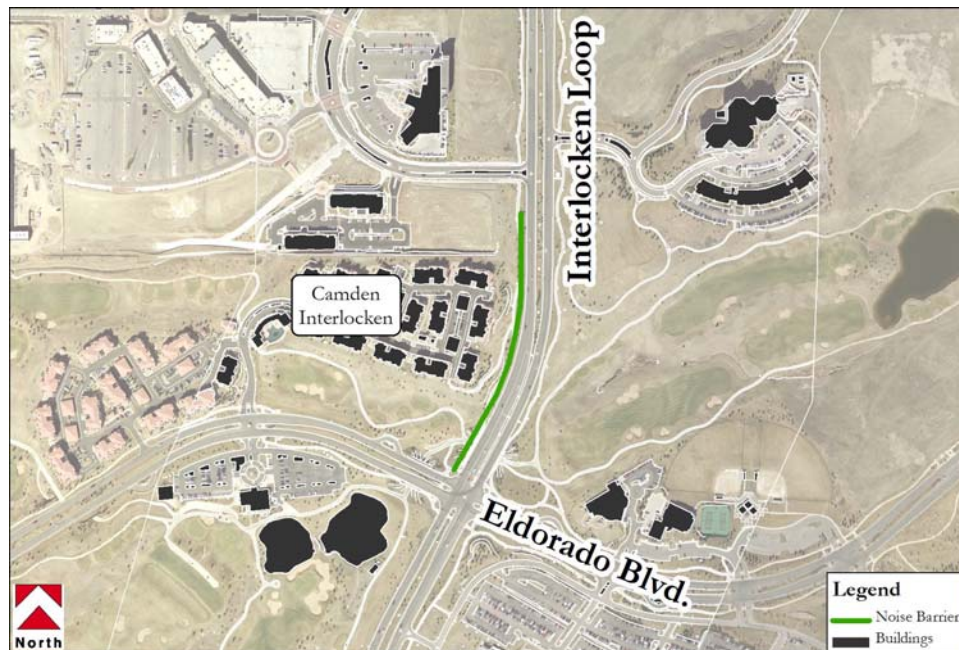
Figure 4.7-12 Recommended Noise Barrier near Camden Interlocken
