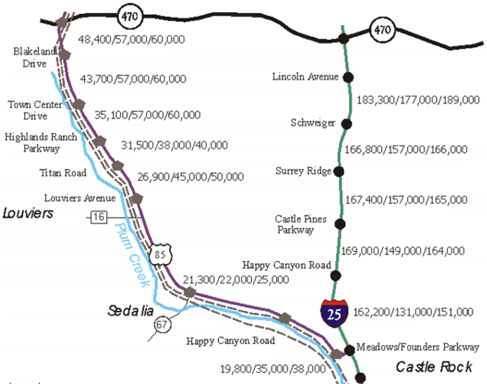
Figure 3.2 2020 Forecasted Average Daily Traffic Model Comparisons South I-25 Corridor and US 85 Corridor/Douglas County Low/Douglas County Moderate
