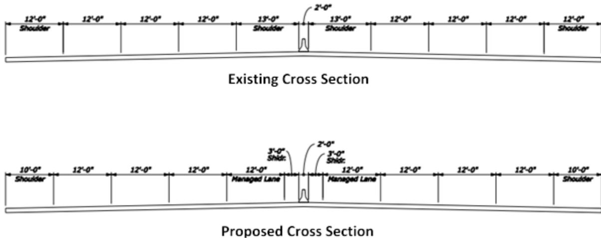
**Figure 4: Typical Cross Section for North I-25 Express Lanes Extension**
