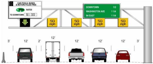
Figure 1: Typical Cross Section of I-35W Priced Dynamic Shoulder Lane (Mn/DOT, 2008).
