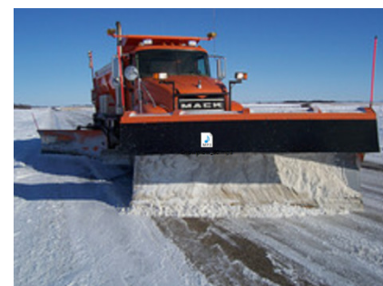
Snow removal equipment would need to either be retrofitted or new equipment purchased to accommodate snow removal for both the Reversible Lane and I-70 operations due to narrow lane width.
