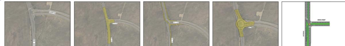
No Action At-Grade Intersection Improvements Grade Separated Turning Movement Roundabout Channelized-T Intersection
