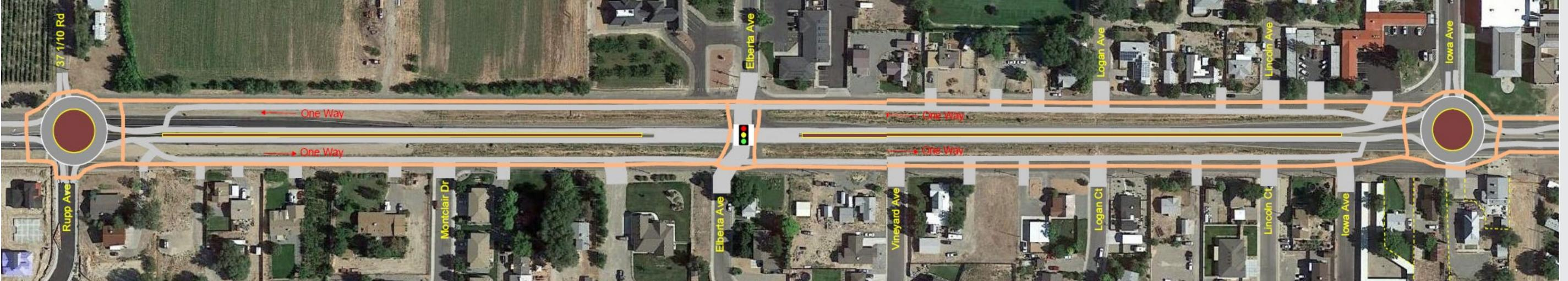
Eliminated in first tier of screening — A traffic signal is not warranted and does not provide the same safety benefits as roundabouts.
