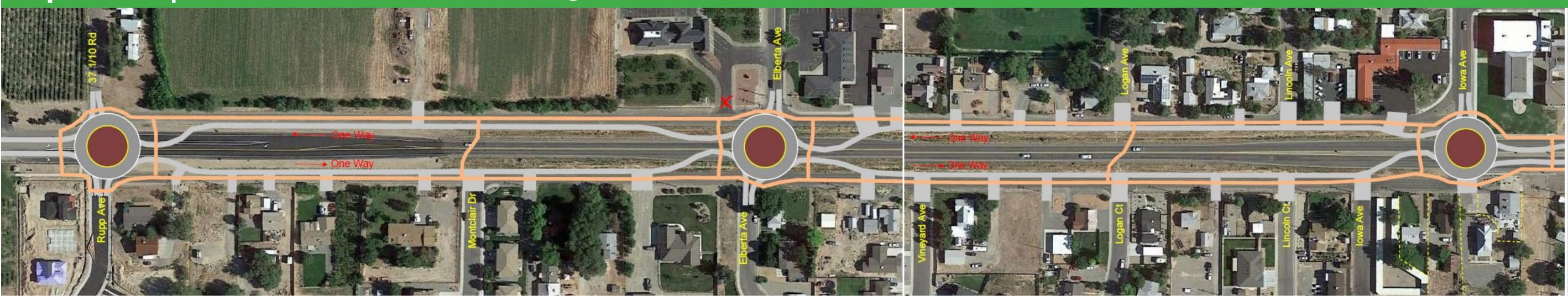
Eliminated in first tier of screening — Does not effectively manage the multiple private access points to US 6, concern with backing onto US 6 from driveways.
