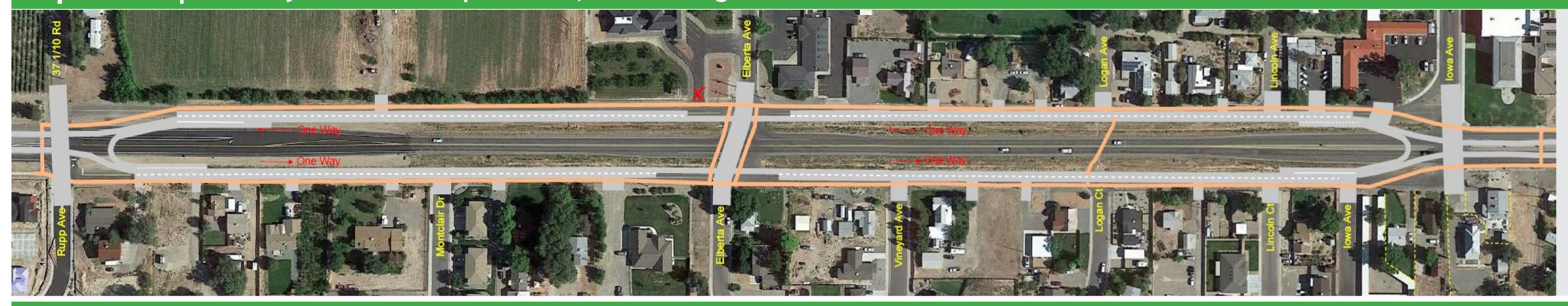
Eliminated in first tier of screening — Does not effectively manage the multiple private access points to US 6. Stop sign control is not desired.
