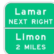
Ground-Mounted Supplemental (Interstates/Freeways)
