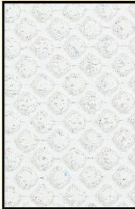
**Figure 3.** Type III Preformed Plastic Tape
