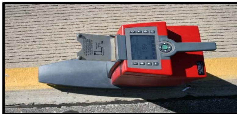
**Figure 8.** Handheld Reflectometer
