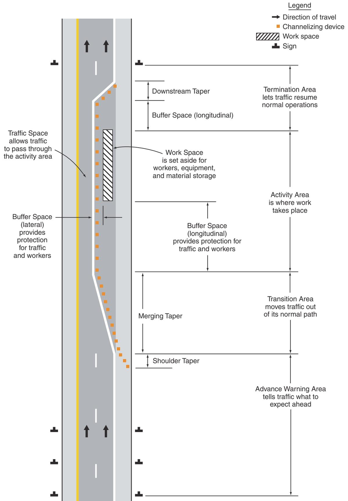
Figure 1. Traffic Space, Work Space, and Buffer Spaces.<sup>1</sup>
