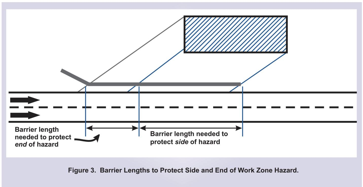
**Figure 3. Barrier Lengths to Protect Side and End of Work Zone Hazard.**
