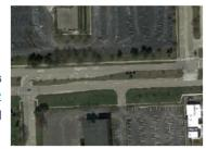
Offset-T Intersection: The minor street is bifurcated at the major roadway at two Tintersections, whereas through movements on the minor roadway use a portion of the major street between intersections. The minor street can be either offset right (as pictured above) or offset left, and the intersections can be unsignalized or signalized. If signalized, proper signal coordination is essential for efficient
