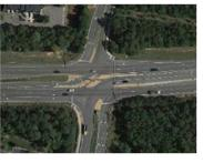
Superstreet / Reduced Conflict Intersection: Similar to the Median U-turn but features break in cross-street traffic that allows signals on opposite directions to operate independently. Left turns can make direct turns onto the minor road but minor road thru and left turn movements are made using the directional U-turn crossovers. A Superstreet / RCI has 14 baseline conflict points (over 3 intersections).
