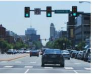
Signalized Intersection: The most common ype of signalized intersection with high driver amiliarity. Signal could be simple two-phase or more complex 8-phase to serve vehicular demand. Left turns can be permitted or protected (or combination of both). At a conventional 4-leg intersection there are 32 baseline conflict points.
