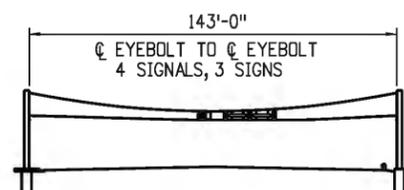
SELECT THE STRAIN POLE SIZE, SPAN-WIRE DIAMETER, AND CAISSON DEPTH FOR A SINGLE SPAN INSTALLATION FOUNDED IN COHESIONLESS SOIL AS SHOWN ABOVE.
