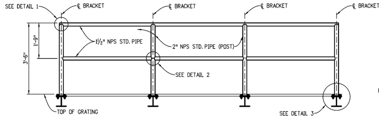
**SAFETY RAILING ELEVATION**
