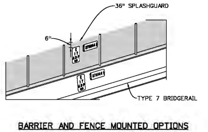
WALL AND MINOR STRUCTURE IDENTIFICATION PANELS
