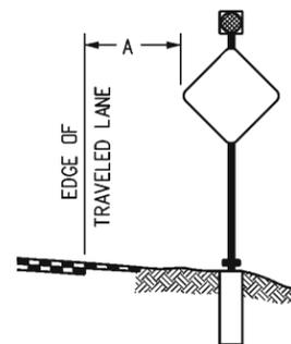
NORMAL LATERAL PLACEMENT "A" FOR WARNING SIGNS IS 12' PLUS CURB OR SHOULDER WIDTH.
