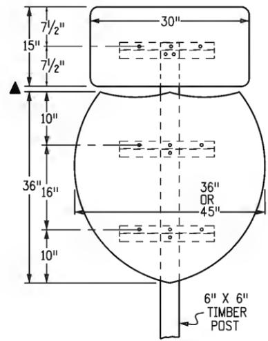
FOR SINGLE POST SIGNS WITH TWO BACKING ZEES, USE ONE 5/8" MACHINE BOLT WITH WASHER AND HEX NUT AND LOCK WASHER AT EACH ZEE.
