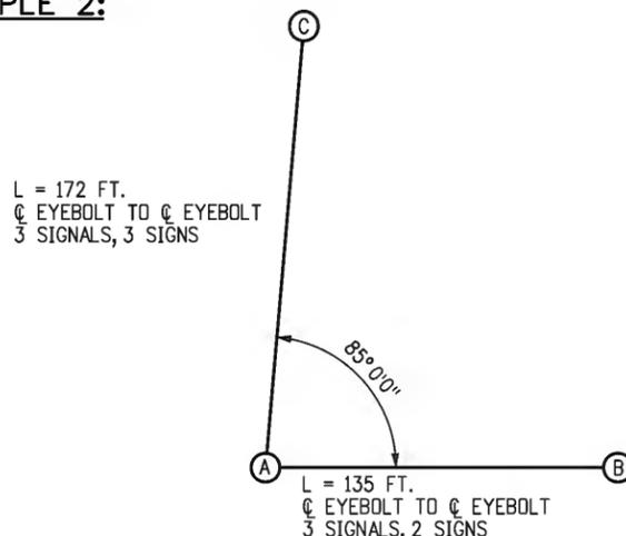
SELECT THE STRAIN POLE SIZES, SPAN-WIRE DIAMETERS, AND CAISSON DEPTHS FOR A DOUBLE SPAN (L-PLAN BOX) FOUNDED IN COHESIVE SOIL AS SHOWN ABOVE.
