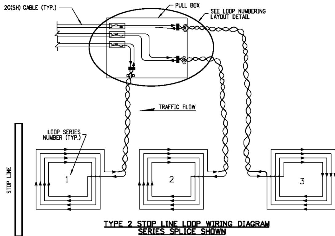
**TYPE 2 STOP LINE LOOP WIRING DIAGRAM
