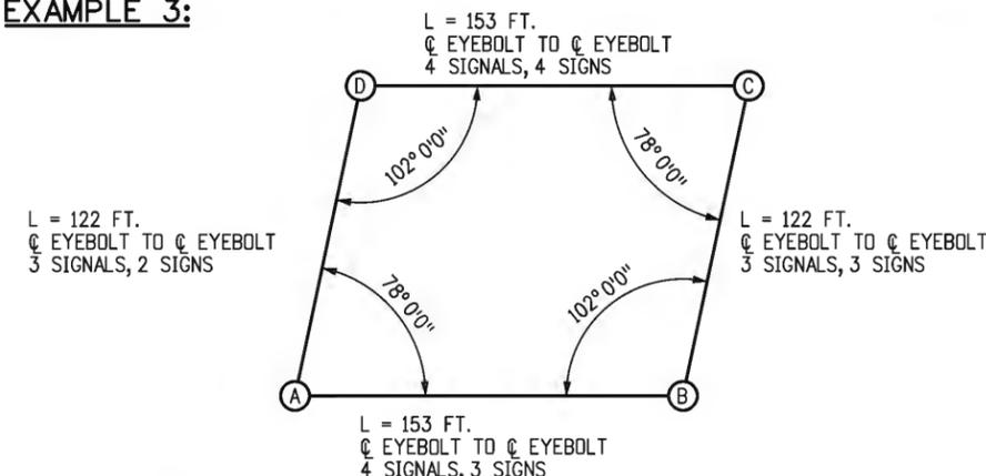
SELECT THE STRAIN POLE SIZES, SPAN WIRE DIAMETERS AND CAISSON DEPTHS FOR CAISSONS FOR A DOUBLE SPAN (RECTANGULAR PLAN BOX) FOUNDED IN COHESIONLESS SOIL AS SHOWN ABOVE.
