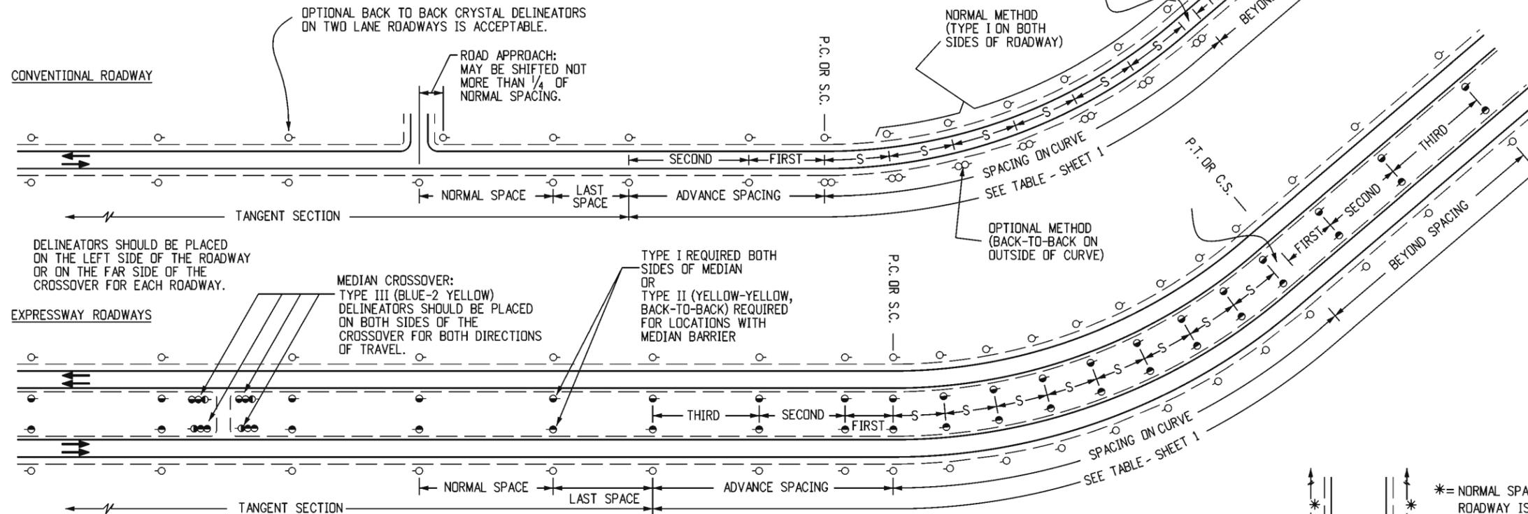
**TYPICAL INSTALLATION FOR TANGENT SECTION AND CURVES**
