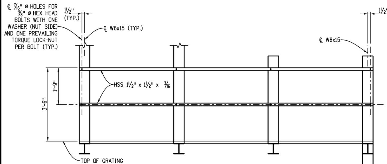
**SAFETY RAILING ELEVATION**
