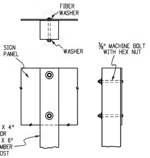
**CLASS I MARKER ASSEMBLY INSTALLATION**
