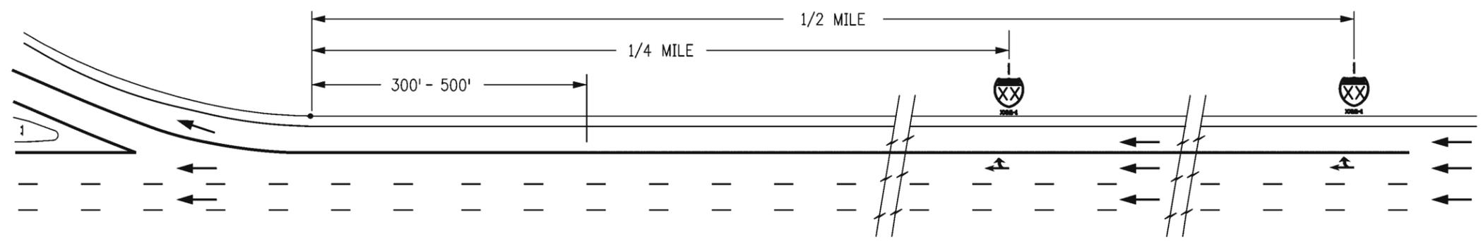
TYPICAL SHIELD & OPTION ARROW PAVEMENT MARKING PLACEMENT
