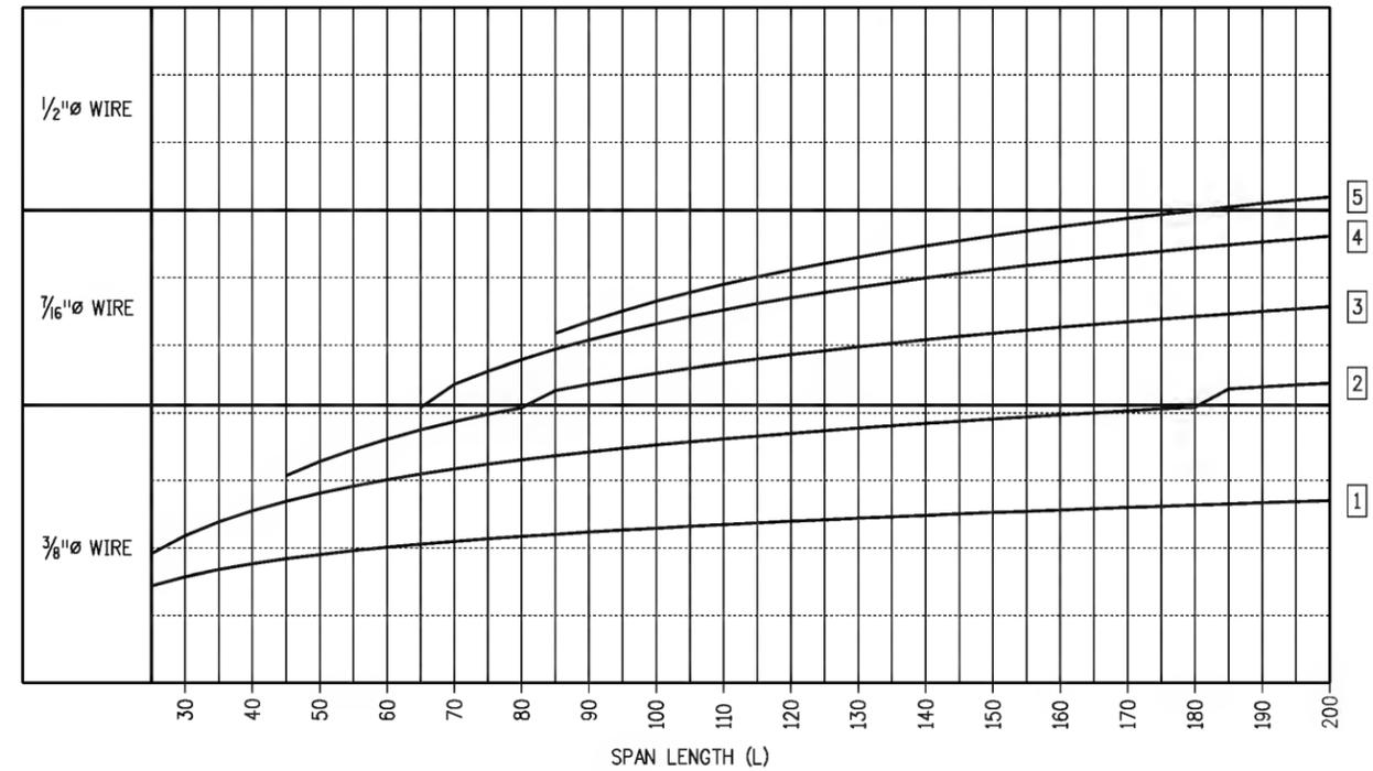
DOUBLE SPAN SPAN-WIRE DIAMETER SELECTION CHART FOR 16" Ø XS POLE
