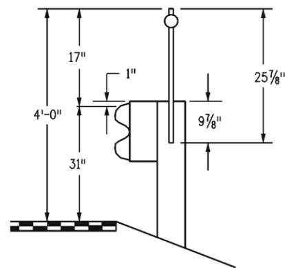
TYPICAL GUARDRAIL POST MOUNT DELINEATORS
