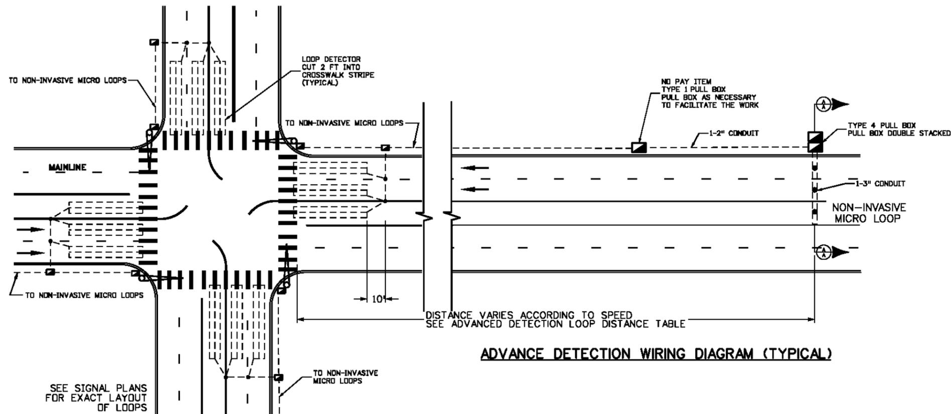
**ADVANCE DETECTION WIRING DIAGRAM (TYPICAL)**
