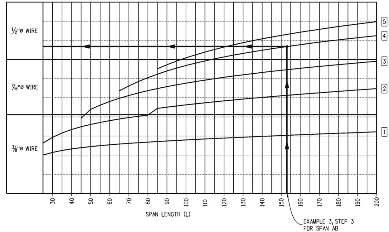
DOUBLE SPAN SPAN-WIRE DIAMETER SELECTION CHART FOR 24" Ø SCH 40 POLE
