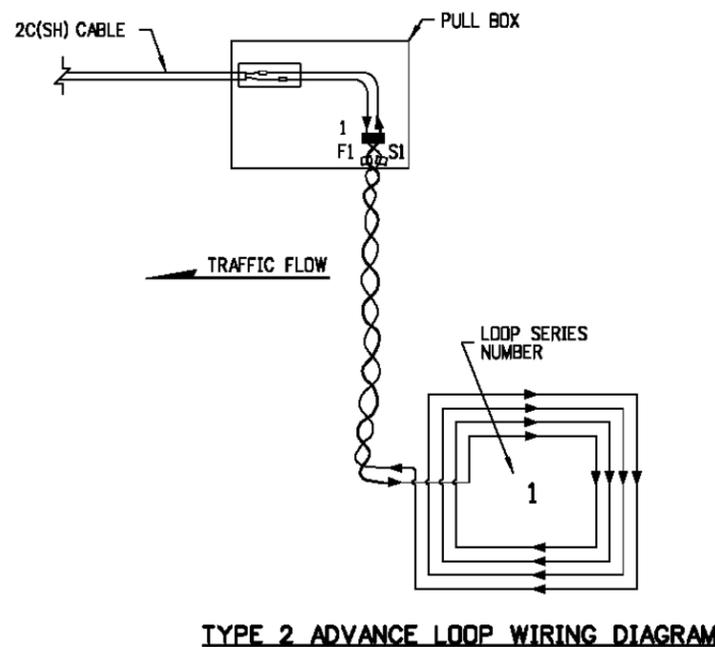
**TYPE 2 ADVANCE LOOP WIRING DIAGRAM**
