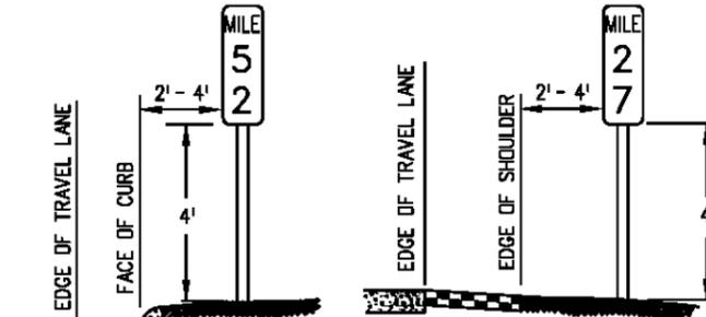
NOTE: MILE MARKERS SHALL BE LOCATED IN LINE WITH DELINEATOR POSTS.
