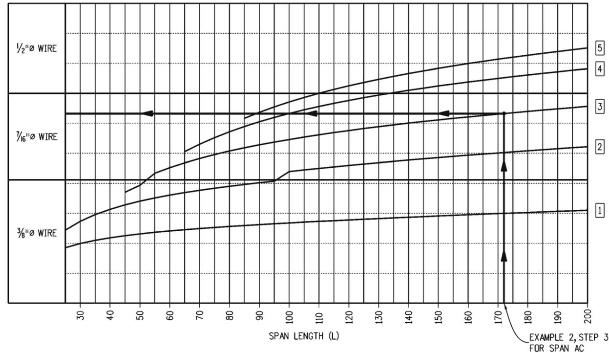
DOUBLE SPAN SPAN-WIRE DIAMETER SELECTION CHART FOR 24" Ø XS POLE
