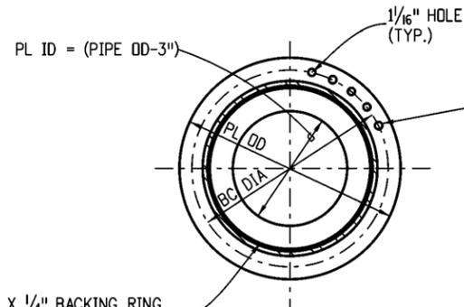
1" Ø H.S. BOLTS (GALVANIZED) EQUALLY SPACED. BOLTS SHALL BE SEQUENTIALLY TIGHTENED. ASSUMING 12 BOLTS AND A CLOCK FACE, THE TIGHTENING SEQUENCE WOULD BE 12, 6, 1, 7 ETC. THIS PROCESS SHALL BE CONTINUED UNTIL NO LOOSE BOLTS ARE FOUND AFTER ALL BOLTS HAVE BEEN INITIALLY TIGHTENED. SEE THE FIELD SPLICE TABLE FOR OTHER DETAILS
