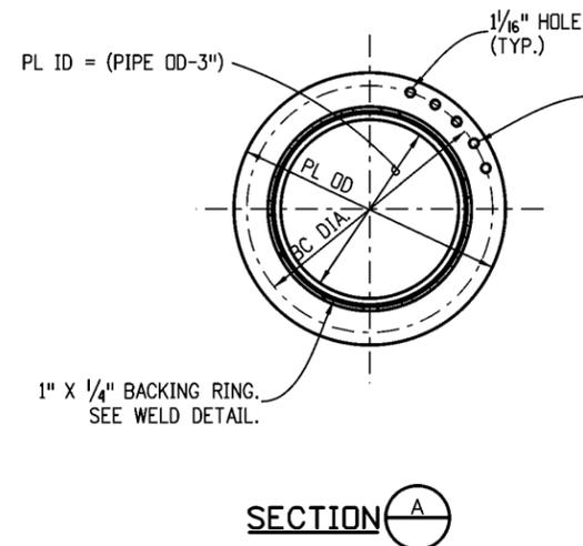
1"  $\varnothing$  H.S. BOLTS (GALVANIZED) EQUALLY SPACED. BOLTS SHALL BE SEQUENTIALLY TIGHTENED. ASSUMING 12 BOLTS AND A CLOCK FACE, THE TIGHTENING SEQUENCE WOULD BE 12, 6, 1, 7 ETC. THIS PROCESS SHALL BE CONTINUED UNTIL NO LOOSE BOLTS ARE FOUND AFTER ALL BOLTS HAVE BEEN INITIALLY TIGHTENED.
