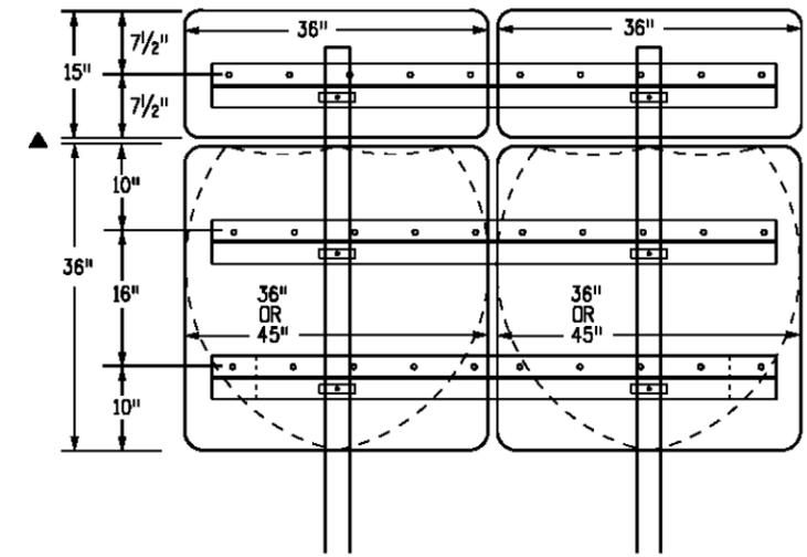
NOTE: THIS CONFIGURATION IS PREFERABLE TO USING TWO SEPARATE SIGNS.
