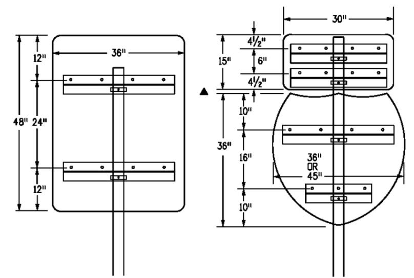
**CLASS II SIGN COMBINATIONS USING T-BRACKETS WITH Z-BAR**
