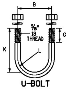
U-BOLT TO BE MADE IN ACCORDANCE WITH STANDARD MANUFACTURING PROCEDURE. 1/4" OR 5/16" DIAMETER STOCK IS PERMISSIBLE. AMERICAN STANDARD REGULAR SEMI-FINISHED HEX NUTS AND SPRING LOCKWASHERS.
