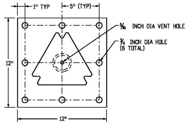
**SURFACE MOUNT SLIPBASE BASE PLATE FABRICATION REQUIREMENTS**
