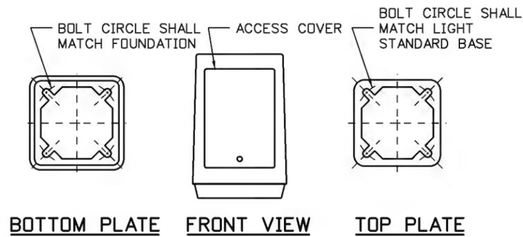
NOTE: MATCH EXISTING BREAKAWAY TRANSFORMER BASE AS CLOSELY AS POSSIBLE.
