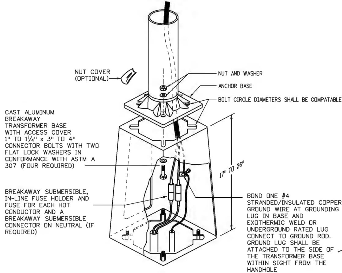
**TYPICAL BREAKAWAY TYPE TRANSFORMER BASE DETAIL**
