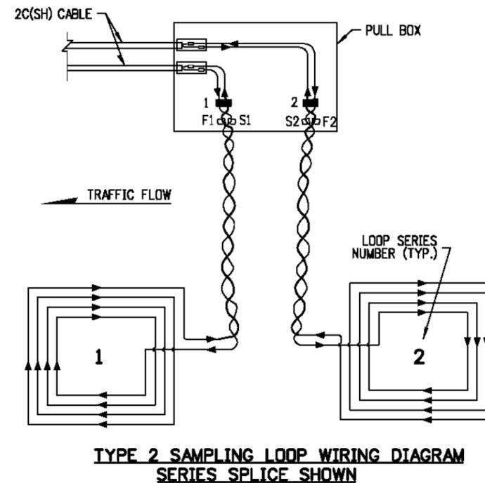
**TYPE 2 SAMPLING LOOP WIRING DIAGRAM
