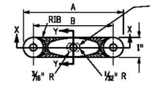
SLOT TO HOLD HEAD OF 3/8" HEX HEAD BOLT. THE BOLT SHALL BE 1 1/4" LONG, WITH FULL THREADS, A MEDIUM WASHER, AND GALVANIZED STEEL OR ALUMINUM SELF-LOCKING HEX HEAD NUT. THE BOLT HEAD MUST NOT TURN IN THE SLOT.
