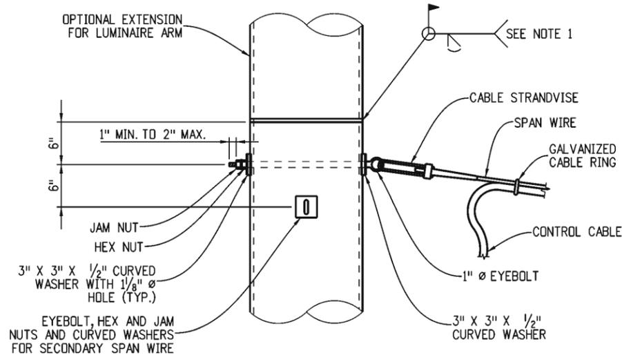
**STRAIN POLE WITH LUMINAIRE ARM EXTENSION**
