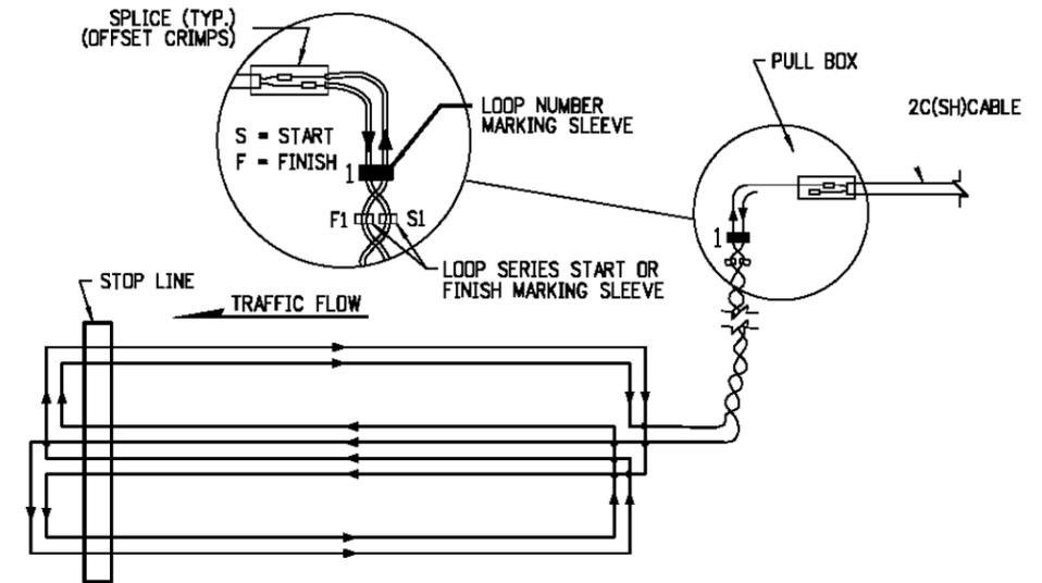
**TYPE 1 STOP LINE LOOP WIRING DIAGRAM**
