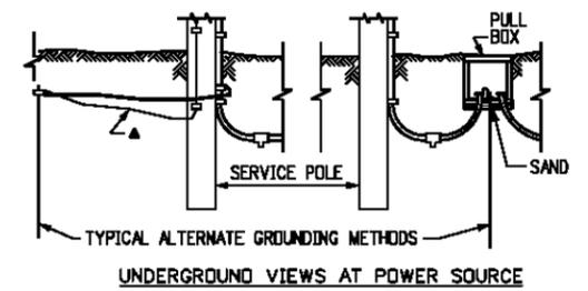
**TYPICAL ALTERNATE GROUNDING METHODS UNDERGROUND VIEWS AT POWER SOURCE**
