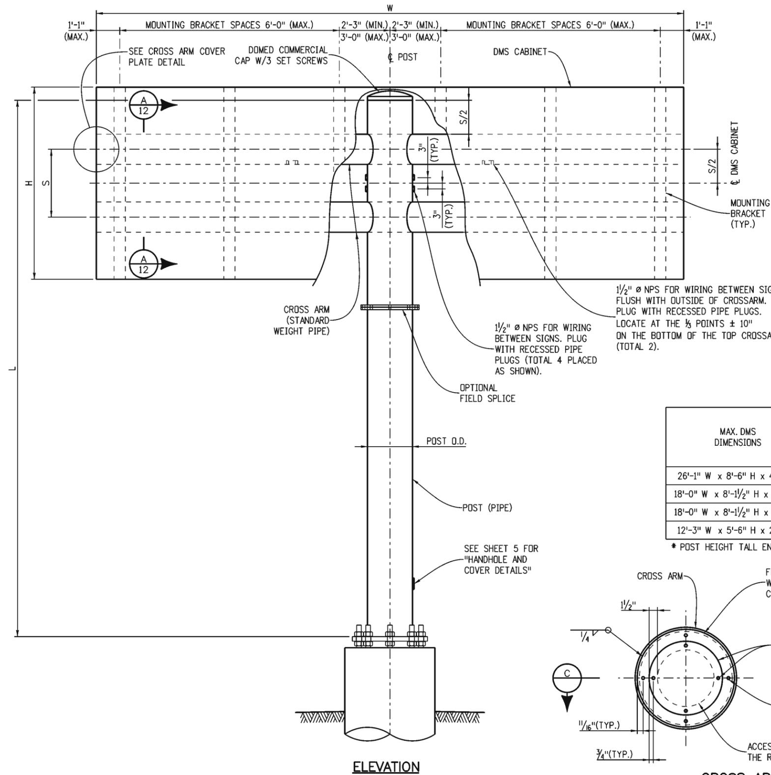
7/8" Ø x PIPE O.D. + 2" A307 BOLT w/ WASHER & JAM NUT (TYP.)
