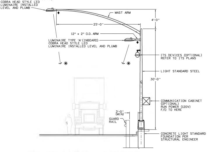
TYPICAL CHAIN STATION TWIN HEAD ASSEMBLY LIGHT STANDARD STEEL (30-FOOT) (SPECIAL) (2 ARM) NOT TO SCALE
