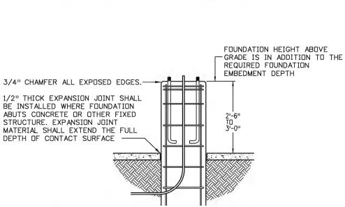
LIGHT STANDARD SUPPLIED. ♦ 2. CONCRETE SHALL BE CLASS 'B' AND SHALL CONFORM TO SECTION 601 FOR CONCRETE AND SECTION 602 FOR REINFORCING STEEL.
