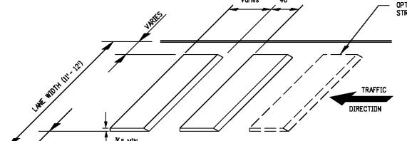
DETAIL - TEMPORARY PORTABLE RUMBLE STRIP ARRAY
