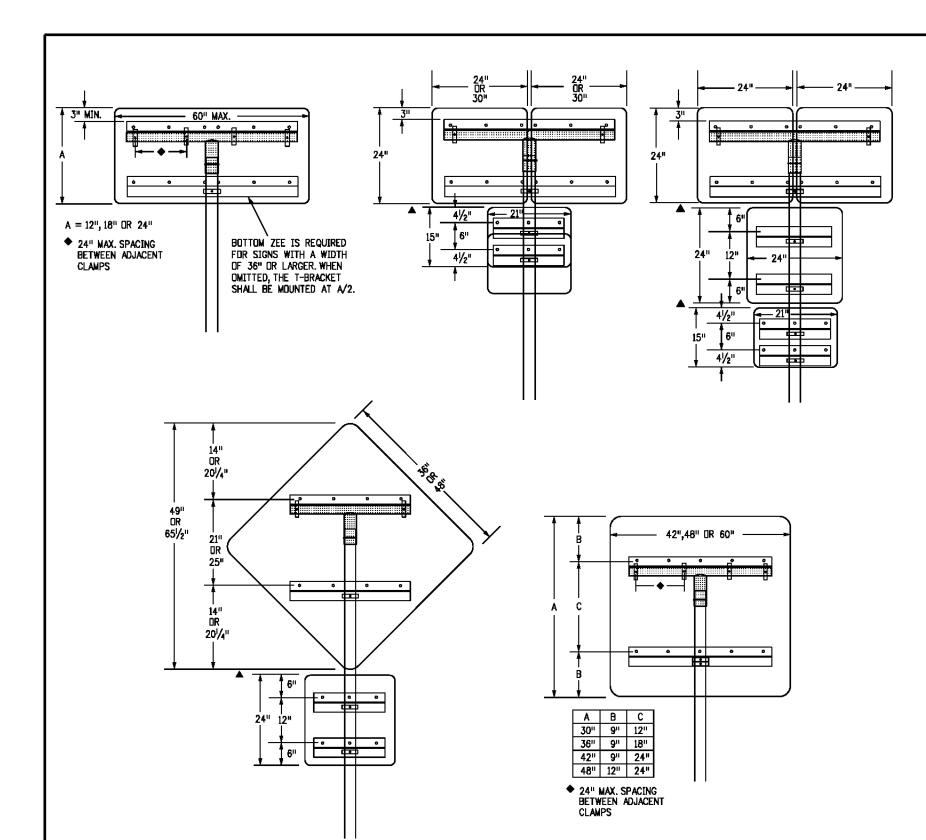
CLASS II SIGN COMBINATIONS USING T-BRACKETS WITH Z-BAR
