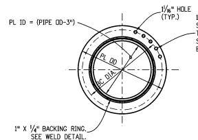
1" Ø H.S. BOLTS (GALVANIZED) EQUALLY SPACED. BOLTS SHALL BE SEQUENTIALLY TIGHTENED. ASSUMING 12 BOLTS AND A CLOCK FACE, -THE TIGHTENING SEQUENCE WOULD BE 12, 6, 1, 7 ETC. THIS PROCESS SHALL BE CONTINUED UNTIL NO LOOSE BOLTS ARE FOUND AFTER ALL BOLTS HAVE BEEN INITIALLY TIGHTENED.
