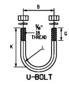
U-BOLT TO BE MADE IN ACCORDANCE WITH STANDARD MANUFACTURING PROCEDURE. 1/4" OR 5/18" DIAMETER STOCK IS PERMISSIBLE. AMERICAN STANDARD REGULAR SEMI-FINISHED HEX NUTS AND SPRING LOCKWASHERS.
