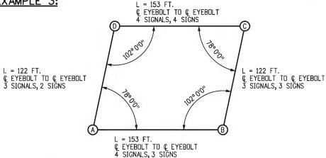
SELECT THE STRAIN POLE SIZES, SPAN WIRE DIAMETERS AND CAISSON DEPTHS FOR CAISSONS FOR A DOUBLE SPAN (RECTANGULAR PLAN BOX) FOUNDED IN COHESIONLESS SOIL AS SHOWN ABOVE.
