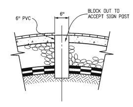
TYPICAL SLEEVE INSTALLATION FOR MEDIAN DELINEATOR POSTS
