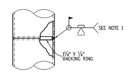
STRUCTURAL WELDED SPLICE
