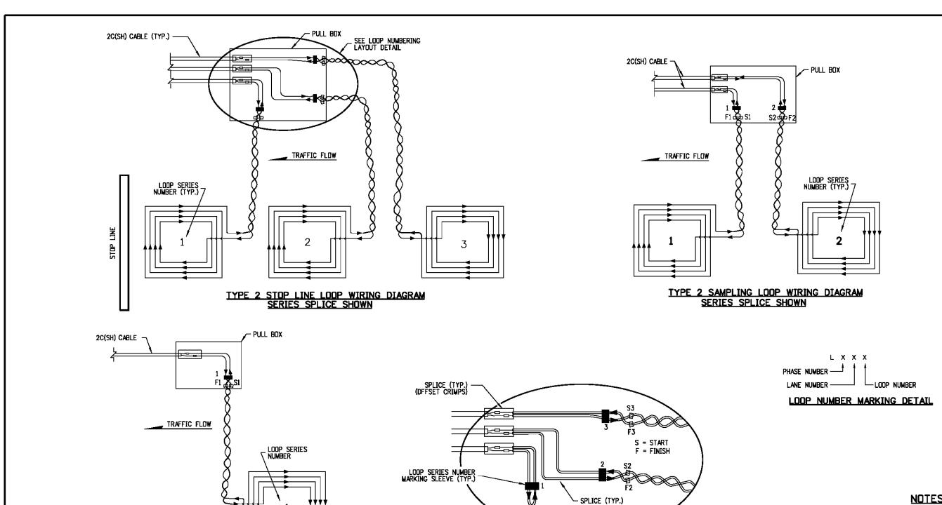
LOOP SERIES START OR FINISH MARKING SLEEVE (TYP.)
