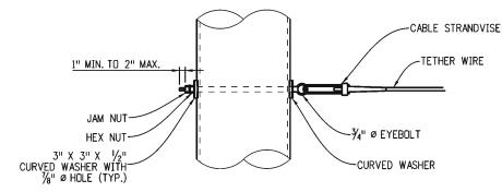
TETHER WIRE CONNECTION TO STRAIN POLE
