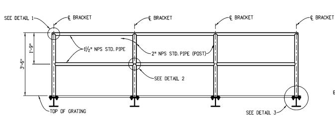
SAFETY RAILING ELEVATION
