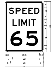
R2-1; 2.3" Radius, 0.9" Border, 0.6" Indent, Black on White; "SPEED", E, "LIMIT", E; "65", E;
