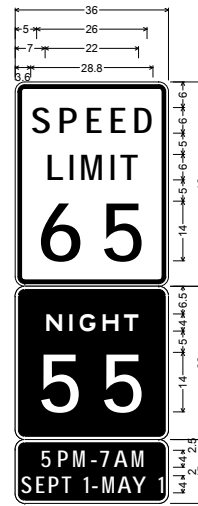
R2-1; 2.3" Radius, 0.9" Border, 0.6" Indent, Black on White; "SPEED" E; "LIMIT" E; "65" E; R2-3P; 2.3" Radius, 0.8" Border, White on Black; "NIGHT" F 150% spacing; "55" E; R2-3a; 2.3" Radius, 0.8" Border, White on Black; "5PM-7AM" D; "SEPT 1-MAY 1" D 70% spacing;
