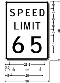
R2-1; 2.3" Radius, 0.9" Border, 0.6" Indent, Black on White; "SPEED" E; "LIMIT" E; "65" E;
