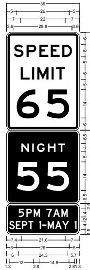
R2-1; 2.3" Radius, 0.9" Border, 0.6" Indent, Black on White; "SPEED", E, "LIMIT", E; "65", E; R2-3P; 2.3" Radius, 0.8" Border, White on Black; "NIGHT", F 150% spacing; "55", E; R2-3a; 2.3" Radius, 0.8" Border, White on Black; "5PM-7AM", D; "SEPT 1-MAY 1", D 70% spacing;
