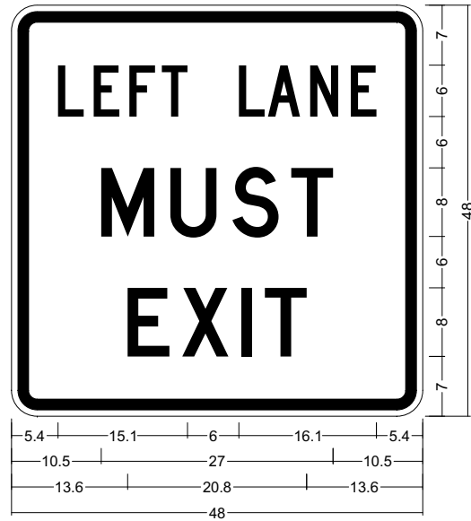
R3-7aL; 3.0" Radius, 1.3" Border, 0.8" Indent, Black on White; "LEFT LANE", C 115% spacing; "MUST", D; "EXIT", D; Table of letter and object lefts
