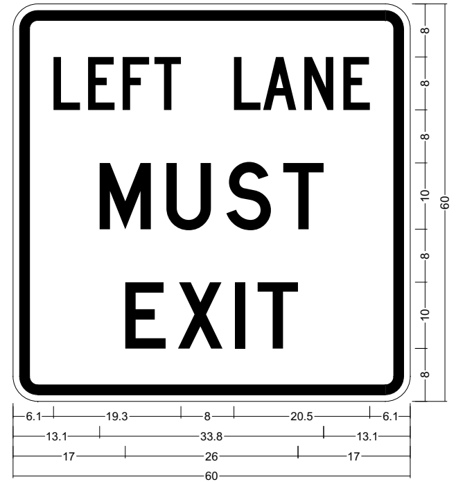
R3-7aL; 3.8" Radius, 1.5" Border, 1.0" Indent, Black on White; "LEFT LANE", C 90% spacing; "MUST", D; "EXIT", D; Table of letter and object lefts
