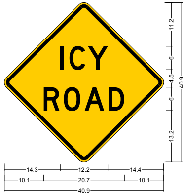
30_W8-50; 30.0" across sides 1.9" Radius, 0.8" Border, 0.5" Indent, Black on Yellow; "ICY", D: "ROAD", D; Table of letter and object lefts
