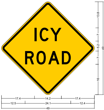
36_W8-50; 36.0" across sides 2.3" Radius, 0.9" Border, 0.6" Indent, Black on Yellow; "ICY", D: "ROAD", D; Table of letter and object lefts
