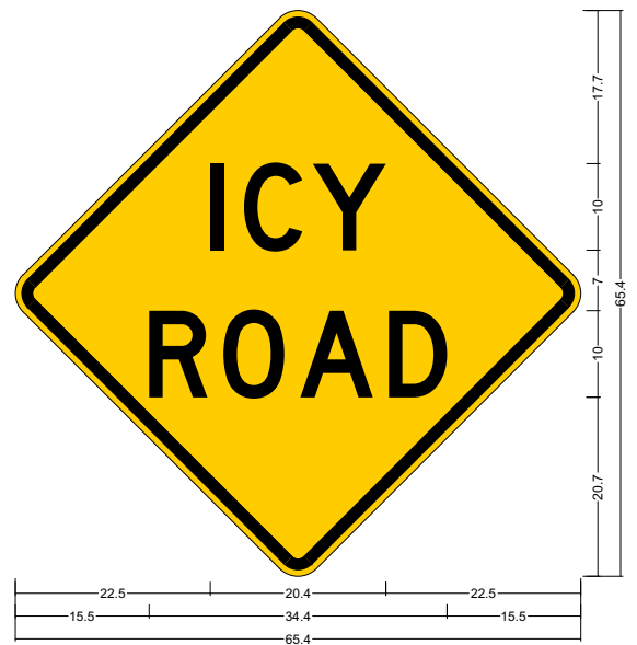
48_W8-50; 48.0" across sides 3.0" Radius, 1.3" Border, 0.8" Indent, Black on Yellow; "ICY", D: "ROAD", D; Table of letter and object lefts
