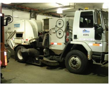
A vacuum sweeper used to remove sand and salt and meet PM 10 (air quality) requirements. The Denver metro area has five vacuum sweepers.
