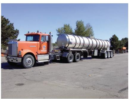
A 6000-gallon tanker used on I-25, I-70, US 36, US 6 and C-470 to spray liquid de-icers. The Denver metro area has three of these tankers.
