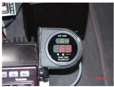
Temperature sensors help maintenance crews determine which product to use. Each plow contains a temperature sensor and maintenance crews frequently verify ambient and pavement temperature throughout the snow removal process.
