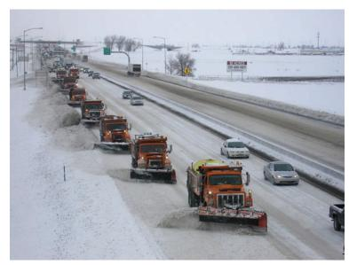
Crews in the Denver metro area often plow in tandem or "gang plow." CDOT performs this maneuver to pull snow and ice away from areas such as walls and medians where drainage is poor. This helps prevent the freeze/thaw cycle that contributes to ice in the driving lanes. Crews make every attempt to accomplish this during low traffic conditions in daylight or near dawn to increase the effectiveness of the de-icing products that are being applied as our crews plow.
