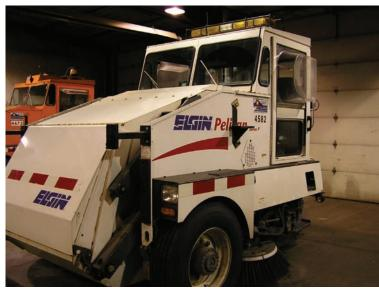
A regular broom used to remove sand and salt and meet PM 10 (air quality) requirements. With this sweeper, the material is swept up and later discarded. The Denver metro area has 12 regular brooms.
