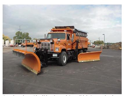
A tandem plow with a V-box for applying solid de-icers and a plow on the front and side to increase plowing activities without increasing manpower or equipment needs. CDOT has 18 tandems with wings in the Denver metro area.
