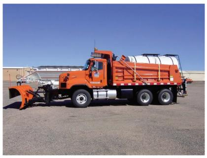
A tandem plow with a 1,600-gallon liquid tank for applying liquid de-icers. CDOT has 42 tandems in the metro area, some have V-boxes for applying solid de-icers and some are combination trucks that can apply both solid and liquid de-icers.
