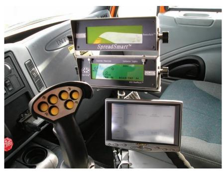
48 CDOT plow trucks in the metro area are equipped with a MDSS touch screen, which allows them to input real-time road and weather information.
