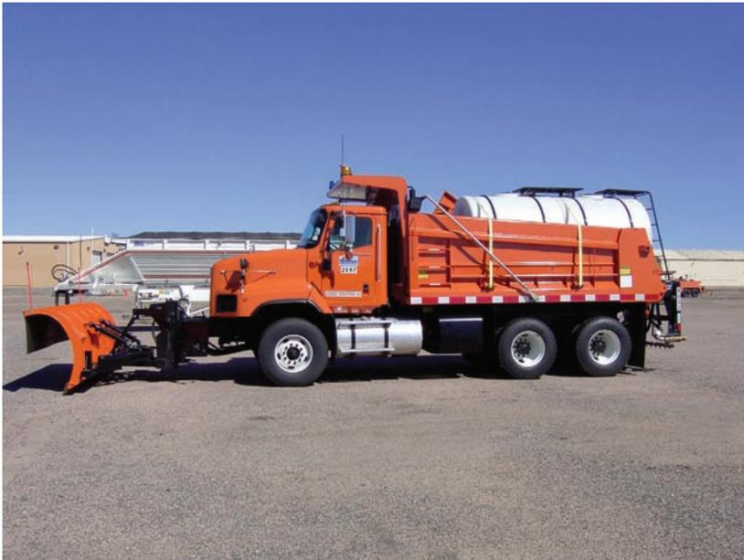
A tandem plow with a 1,600-gallon liquid tank for applying liquid de-icers. CDOT has 42 tandems in the metro area, some have V-boxes for applying solid de-icers and some are combination trucks that can apply both solid and liquid de-icers.
