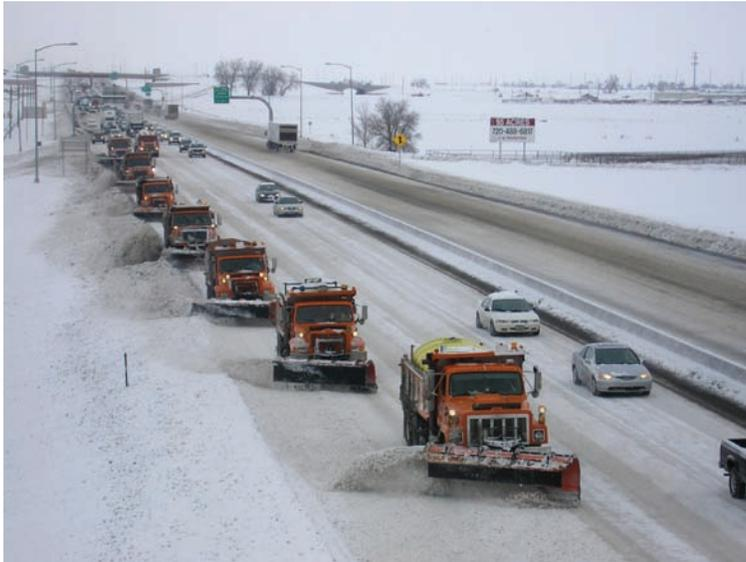
Crews in the Denver metro area often plow in tandem or “gang plow.” CDOT performs this maneuver to pull snow and ice away from areas such as walls and medians where drainage is poor. This helps prevent the freeze/thaw cycle that contributes to ice in the driving lanes. Crews make every attempt to accomplish this during low traffic conditions in daylight or near dawn to increase the effectiveness of the de-icing products that are being applied as our crews plow.
