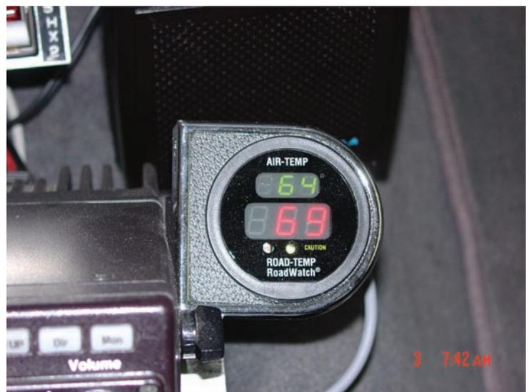
Temperature sensors help maintenance crews determine which product to use. Each plow contains a temperature sensor and maintenance crews frequently verify ambient and pavement temperature throughout the snow removal process.
