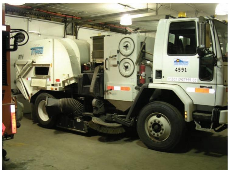
A vacuum sweeper used to remove sand and salt and meet PM 10 (air quality) requirements. The Denver metro area has five vacuum sweepers.
