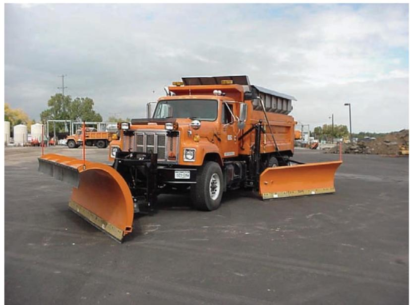
A tandem plow with a V-box for applying solid de-icers and a plow on the front and side to increase plowing activities without increasing manpower or equipment needs. CDOT has 18 tandems with wings in the Denver metro area.
