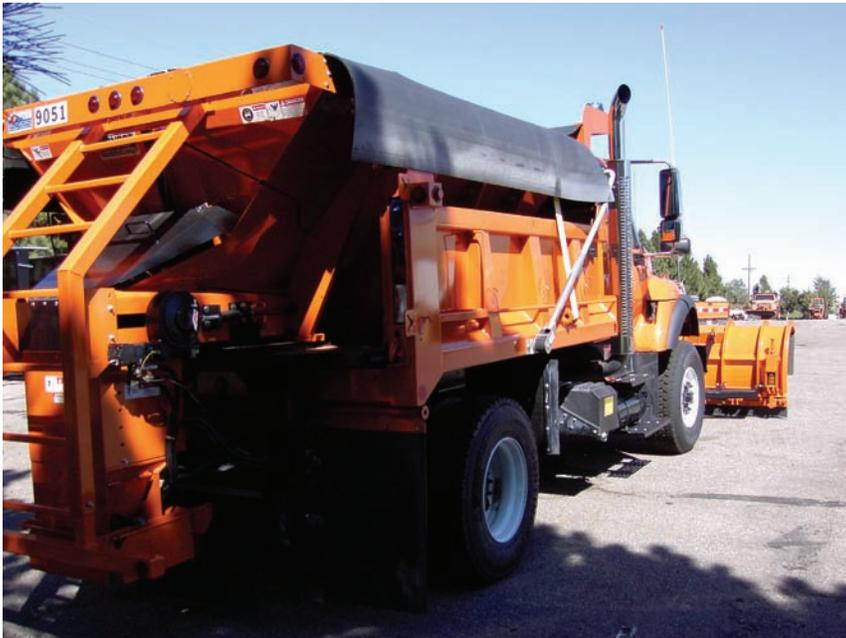
A mid-range plow with a V-box for applying solid de-icers. CDOT has 55 mid-range plows in the Denver metro area. Some of the mid-range plows are equipped with 1,000-gallon tanks for applying liquid de-icers and others are equipped to apply both solid and liquid de-icers.
