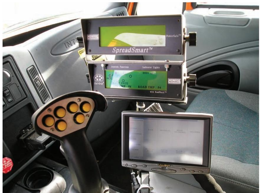
48 CDOT plow trucks in the metro area are equipped with a MDSS touch screen, which allows them to input real-time road and weather information.
